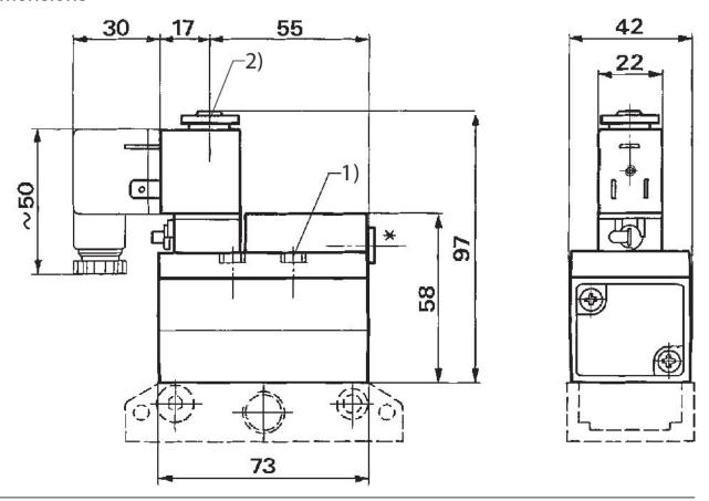
Tightening torque for mounting screws: 2.7 ± 0.3 Nm
