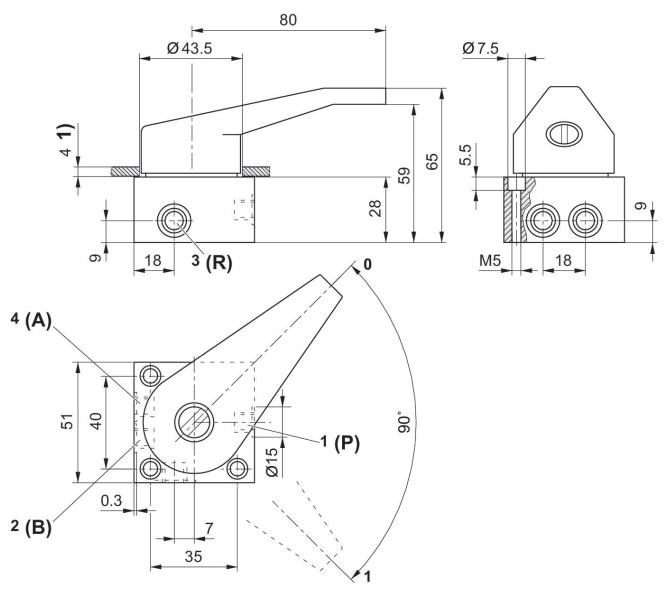
1) Max. Pos. 0: port 1 # port 4, port 2 # port 3 pos. I: port 1 # port 2, port 4 # port 3
