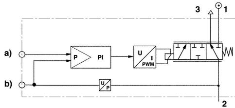
a) Nominal input value b) Actual output value The E/P pressure control valve modulates the pressure corresponding to an analog electrical nominal input value.
