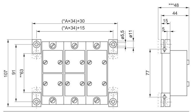
\* A = No. of subbases. \*\* With the mounting holes turned inwards. \*\*\* With the mountings turned 180°.
