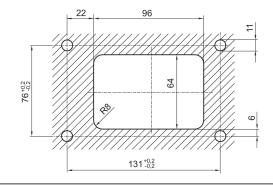
Mounting plate max. 7 mm thick
