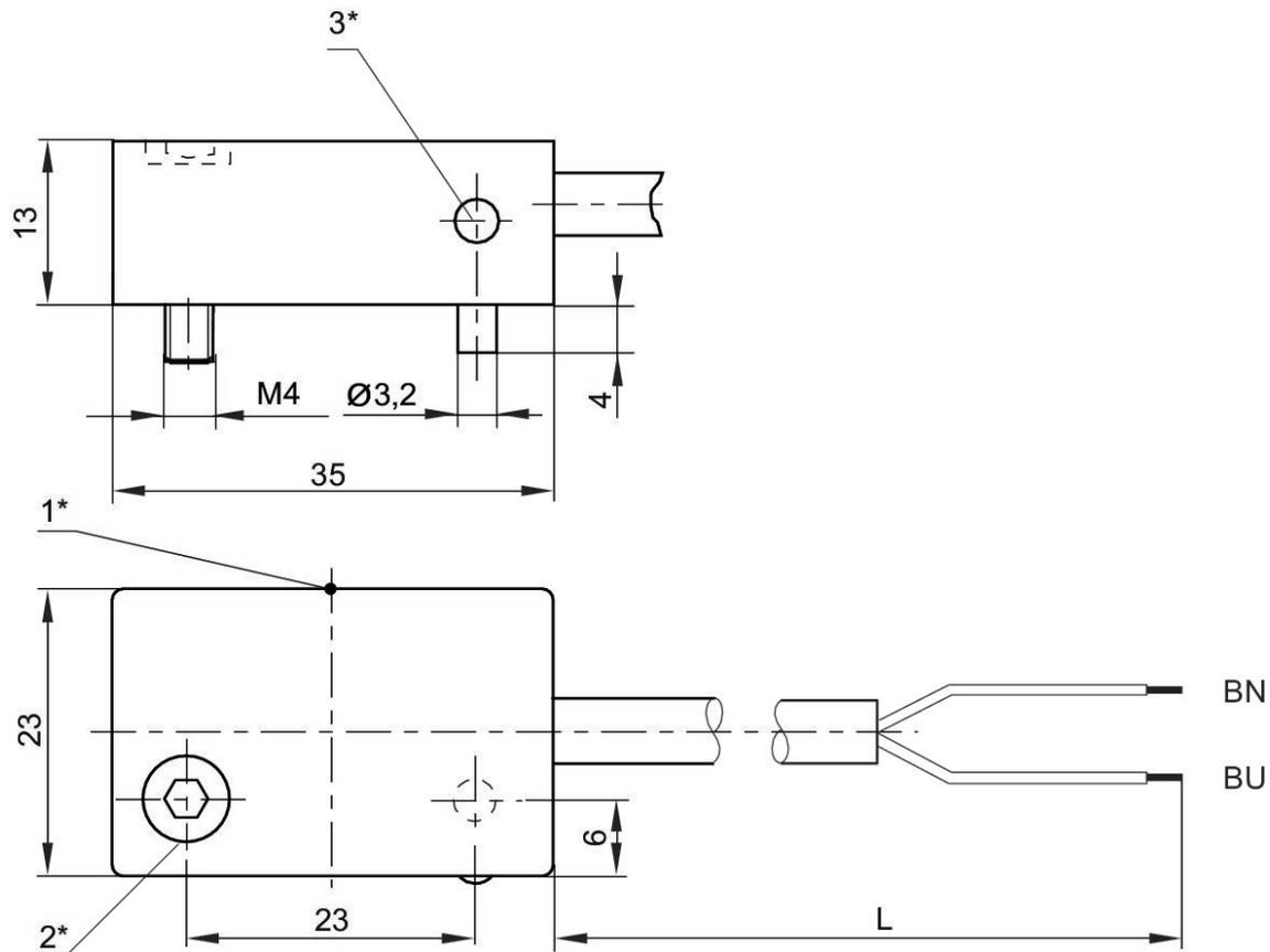
1\* = 开关点 2\* = 紧固螺丝 3\* = LED
