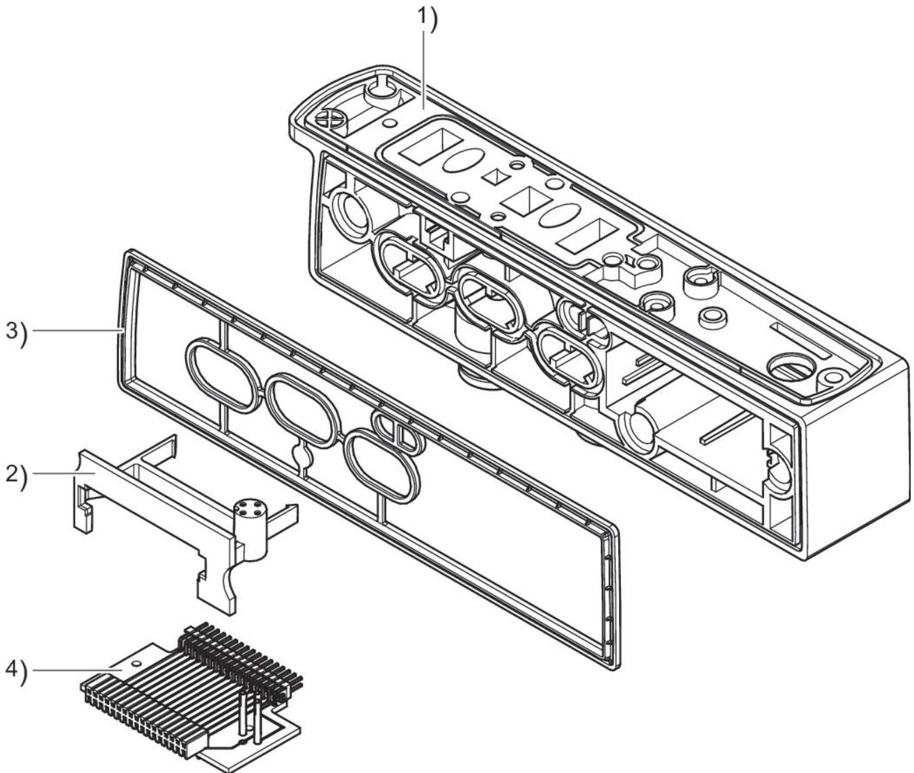
1) Subbase 2) Circuit board holder 3) Seal 4) Circuit board
