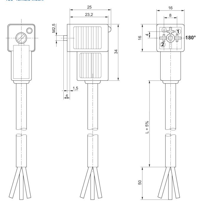
Fig. 1 Dimensions in mm
