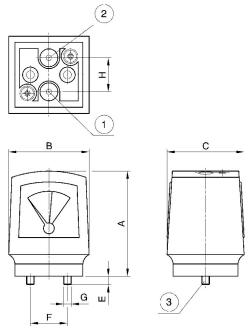
1) Input pressure p1 2) Output pressure p2
