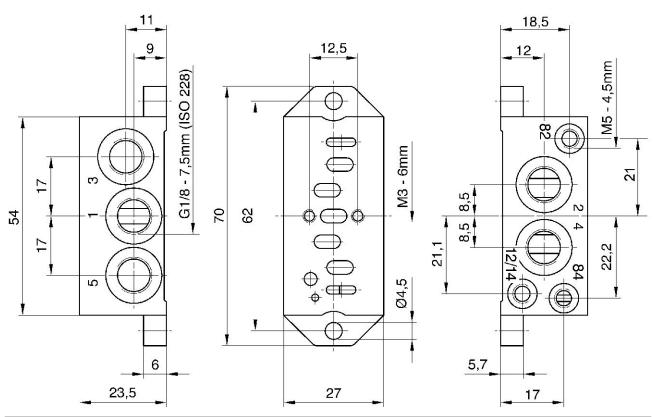
Ports 82 and 84: pilot exhaust air Connection 12 and 14: external pilot
