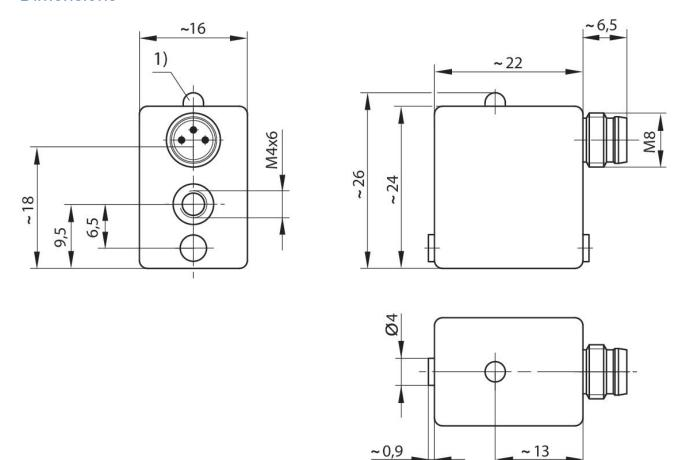
1) LED M8: combination plug can be combined with valve plug connectors Ø6.5 mm and M8.
