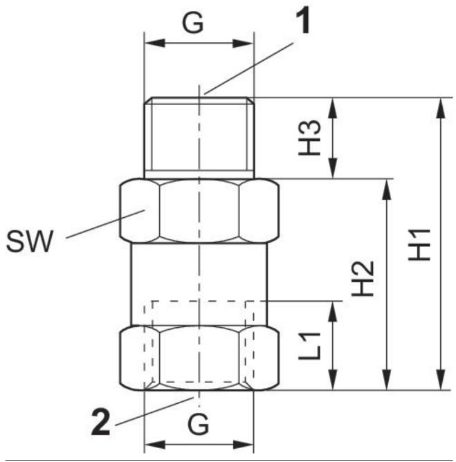
vacuum ejector connection 1, suction cup connection 2
