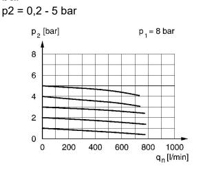
p1 = Working pressure p2 = Secondary pressure qn = Nominal flow
