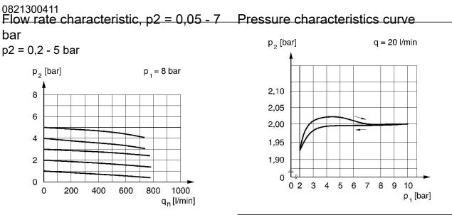
p1 = working pressure p2 = secondary pressure q = flow rate
