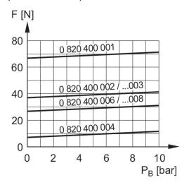
F = actuating force P<sub>B</sub> = Working pressure
