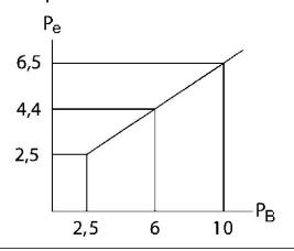
Pe = external control pressure, min.
