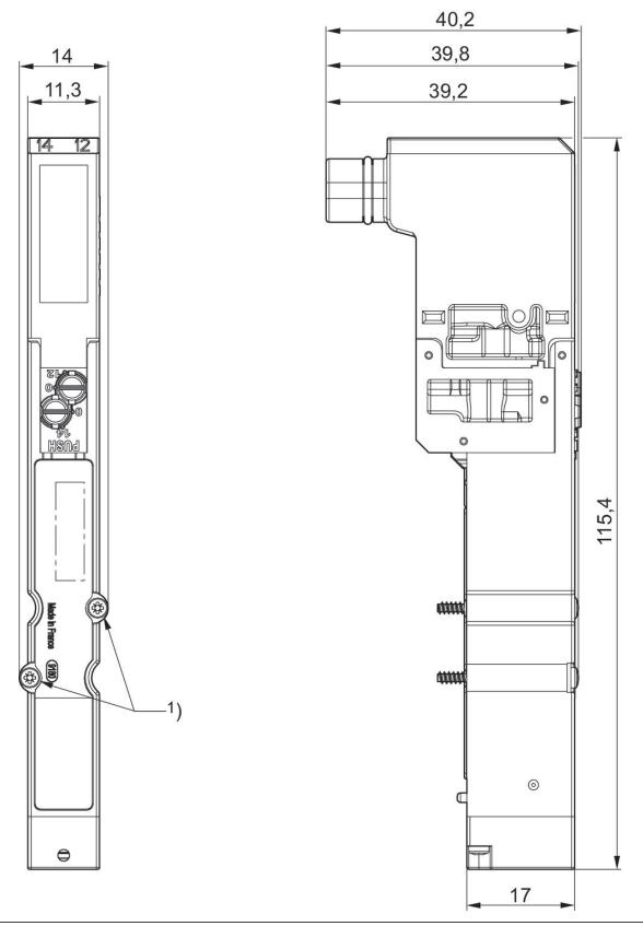
1) Mounting screw: X-slot DIN EN ISO 4757-Z0 tightening torque for mounting screw [Nm]: 0.25
