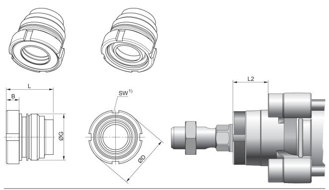
1) Can be mounted with hook wrench in accordance with DIN 1810 A
